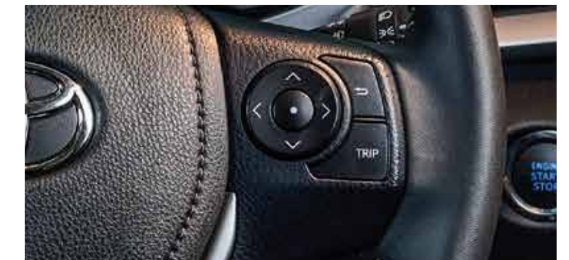
MID CONTROL SWITCHES
